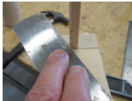
screw the entire frame together. Now, fill your screw holes with wood plugs and trim the excess to flush. Last, fill the 1/4" x 3/8" grooves at the ends of the sides with some leftover scrap from your triangles. A utility knife makes good work for cutting these small pieces. Drop in a bit of glue in the space, set the plug in place and trim to flush. Now, give the frame a quick sand and get ready to harvest some bee-free frames of honey! **BC**
