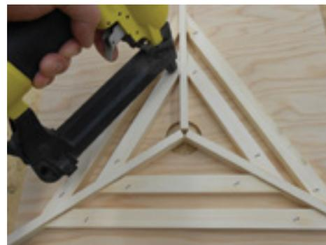
its original position with a few 1/2" staples or nails. Cover the triangles with #8 hardware cloth, secure with staples and trim with metal cutting shears or snips.
