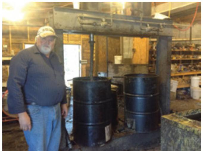
*Tim Trescott and two of the hydraulic wax presses he built using old train pistons.*
