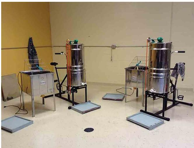
*BeezKneez turned to their bike mechanic, Carl, to convert a broken donated extractor into a pedal-powered dynamo.*
