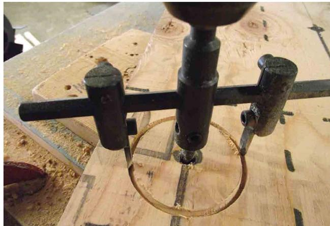
**Caution:** Using a hole cutter like the one pictured can be very dangerous. The bar that holds the cutter heads can fly around at a speed that makes it difficult to see. If your hand or anything else gets in the way, it is guaranteed to hurt.
